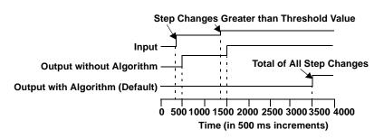
D) If an open sensor is validated at the end of the first update cycle (Time = 500 ms), the output will go directly to alarm level. The original spike (at Time = 0 ms) will not be seen at the output.
